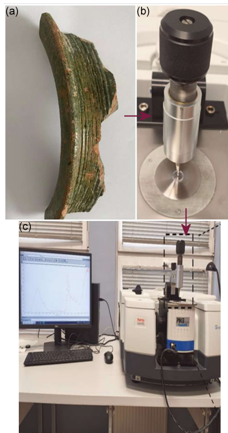
Fig. 4. Sample preparation and FTIR analysis workflow. (a) A 16th-century pottery fragment, (b) fine powdered sample placed on an ATR diamond crystal, and (c) FTIR spectrometer-microscope setup used for measurements.
