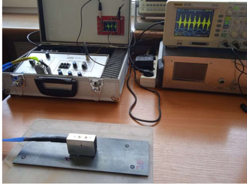
Fig. 3. Laboratory MBN testing equipment for the steel sheet investigations.
