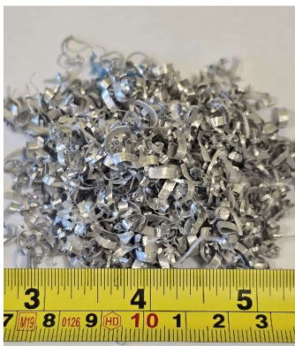
Fig. 2. Material B — chips from machining of EN-AW 5083 alloy.
