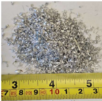
Fig. 3. Material C — chips from machining of EN-AW 5083 alloy.
