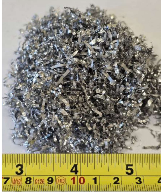
Fig. 1. Material A — chips from machining of EN-AW 5083 alloy.
