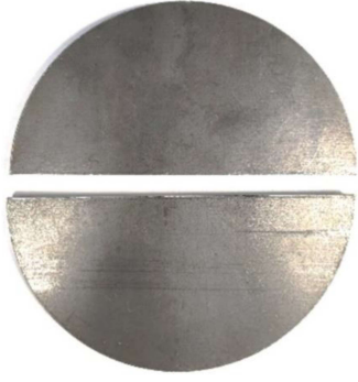
Fig. 2. Semi-finished products after laser cutting operation.
