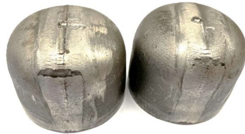
Fig. 9. Defective drawpieces with broken welds.
