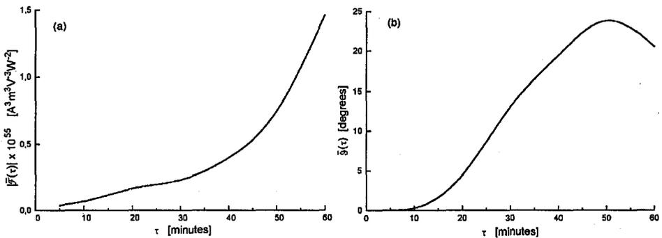
Fig. 2. The absolute value (a) and the angle of rotation in the complex plane (b) of the space-average  $\chi^{(2)}$  encoding function  $\overline{\mathcal{F}}(\tau) = |\overline{\mathcal{F}}(\tau)| \exp[i\overline{\vartheta}(\tau)]$  versus the integral time variable  $\tau$  for the 25 mm long Ge-doped fiber using the data of Lambelet-Feinberg experiment [17].
