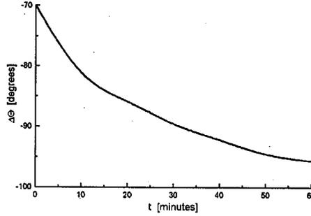
Fig. 1. Time evolution of the mutual phase shift between the SH radiation generated in the fiber and the SH seeding radiation,  $\Delta\Theta = \varphi_{2\omega}^{\text{seed}} - \varphi_{2\omega}^{\text{gen}}$ , using the data of Lambelet-Feinberg experiment [17].
