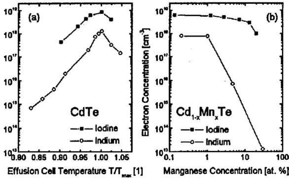
Fig. 1. Room temperature electron concentration in MBE-grown iodine- and indium-doped (a) CdTe and (b)  $\text{Cd}_{1-x}\text{Mn}_x\text{Te}$  layers determined from the Hall measurements.
