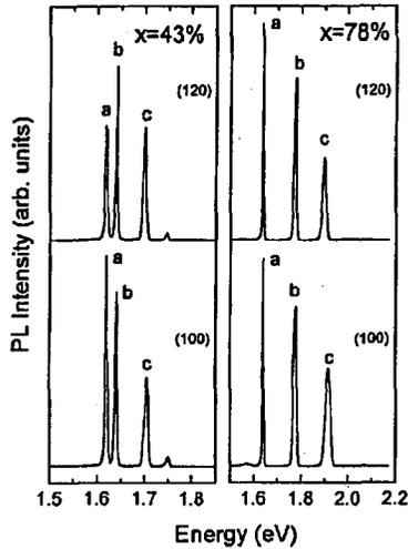
Fig. 1. PL spectra of two pairs of simultaneously grown (100)- and (120)-oriented quantum well structures taken at  $T = 10$  K. Each structure contains three QWs: two regular CdTe QWs with the width 77.8 Å and 19.5 Å labeled *a* and *c*, respectively, and one DMQW ( $3 \times 1$ ) labeled *b*. Compositions of the barriers are given in the figure.
