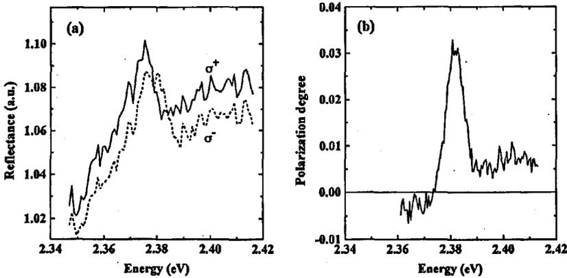
Fig. 1. Reflectance spectra of  $\text{Zn}_{1-x}\text{Fe}_x\text{Te}$ ,  $x \approx 0.002$  (a) and degree of polarization of reflectance  $\mathcal{P}$  (Eq. 3) (b) at  $T = 1.9$  K and magnetic field  $B = 5$  T.
