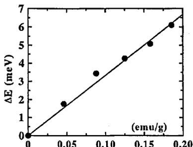
Fig. 2. Exciton splitting  $E(\sigma^-) - E(\sigma^+)$  versus macroscopic magnetization of  $\text{Zn}_{1-x}\text{Fe}_x\text{Te}$ ,  $x \approx 0.002$  at  $T = 1.9$  K. The straight line corresponds to  $N_0\alpha - N_0\beta = 2.1$  eV.
