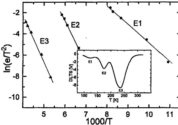
Fig. 1. Arrhenius plots and corresponding thermal DLTS scan (inset in the figure) for the sample *G1*: *n*-type CdMnTe:Ga doped of 1% Mn content.  $U_R = -4$  V,  $U_{p1} = -3$  V,  $U_{p2} = -3.5$  V and filling pulses widths  $t_{p1} = t_{p2} = 50$   $\mu\text{s}$ . The temperature scan presented in the inset was taken for the lock-in frequency  $f = 233$  Hz.
