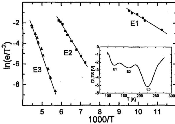
Fig. 3. Arrhenius plots and corresponding thermal DLTS scan (inset in the figure) for the sample *I1*: *n*-type CdMnTe:In doped of 20% Mn content.  $U_R = -4$  V,  $U_{p1} = -3$  V,  $U_{p2} = -3.5$  V and  $t_{p1} = t_{p2} = 0.5 \mu\text{s}$ . The temperature scan was taken for the lock-in frequency  $f = 2500$  Hz.
