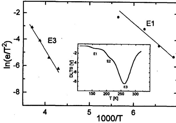
Fig. 2. Arrhenius plots and corresponding thermal DLTS scan (inset in the figure) for the sample *G2*: *n*-type CdMnTe:Ga doped of 5% Mn content.  $U_R = -3$  V,  $U_{p1} = -2$  V,  $U_{p2} = -2.15$  V and filling pulses widths  $t_{p1} = t_{p2} = 5 \mu\text{s}$ . The temperature scan was taken for the lock-in frequency  $f = 500$  Hz.
