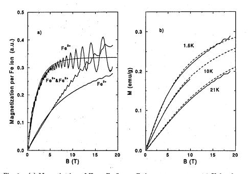
Fig. 1. (a) Magnetization of  $Hg_{1-x}Fe_xSe$  per Fe ion at temperature 4.2 K for three samples labelled as follows:  $Fe^{3+} - x = 0.0002$ ,  $Fe^{2+}$  and  $Fe^{3+} - x = 0.003$ ,  $Fe^{2+} - x = 0.003$ ;  $7 \times 10^{18}$  cm<sup>-3</sup> Ga. Solid lines — experiment, dashed line — Brillouin function j = 5/2; (b) magnetization of  $Hg_{0.997}Fe_{0.003}Se$ ;  $7 \times 10^{18}$  cm<sup>-3</sup> Ga at 1.6, 10, 21 K. Solid lines — experiment, dashed lines — theory.
