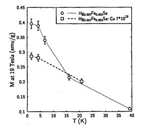
Fig. 2. The absolute value of magnetization taken at 19 T as a function of temperature.
