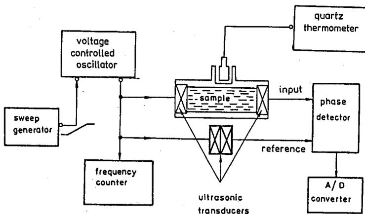
Fig. 2. The measuring setup used for the determination of the absolute value of ultrasonic wave propagation by the phase method, with tunable continuous wave.
