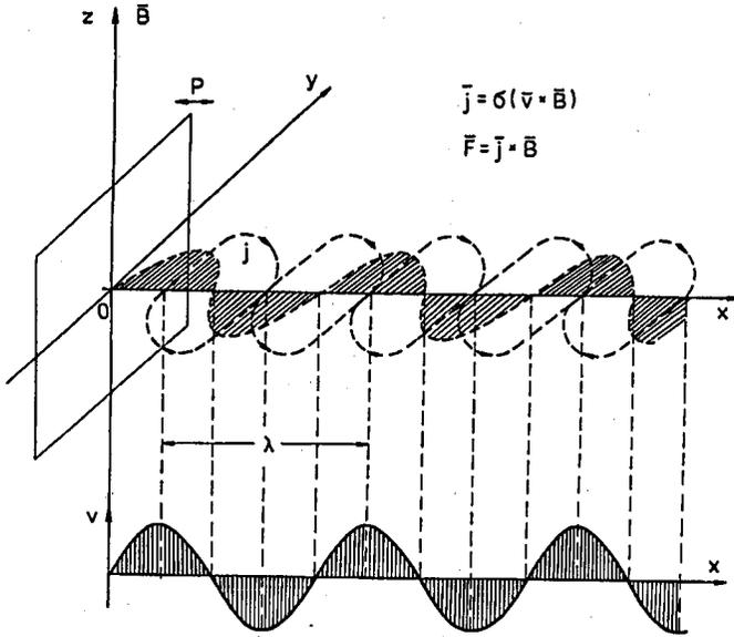
Fig. 1. The induction of eddy currents in an electrically conducting liquid medium in a strong external magnetic field at propagation of an ultrasonic wave in the medium.
