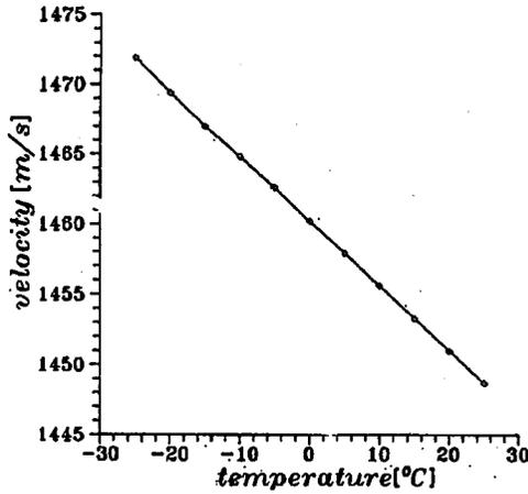
Fig. 5. Ultrasonic propagation velocity in mercury versus temperature, for  $f = 2$  MHz.
