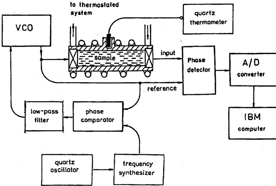
Fig. 3. Setup for the determination of changes in ultrasonic propagation velocity by the phase method.
