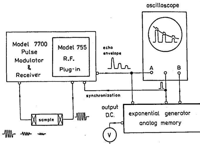
Fig. 4. Block diagram of the setup for measuring the absorption coefficient of ultrasonic waves in mercury.
