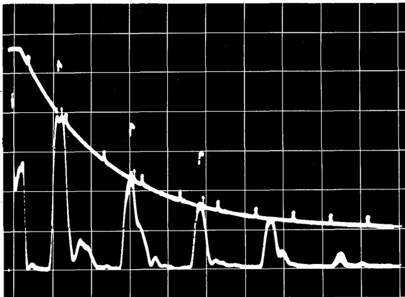
Fig. 7. Picture of the ultrasonic pulses, obtained on the oscilloscope screen, in the absence of magnetic field.
