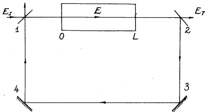
Fig. 1. Ring cavity configuration.
