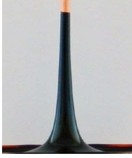
Fig. 5. Example of the shape of the free surface of the ferrofluid surrounded by a wire with radius r = 1.5 mm for current intensity I = 140 A. (Photo made by the author).
