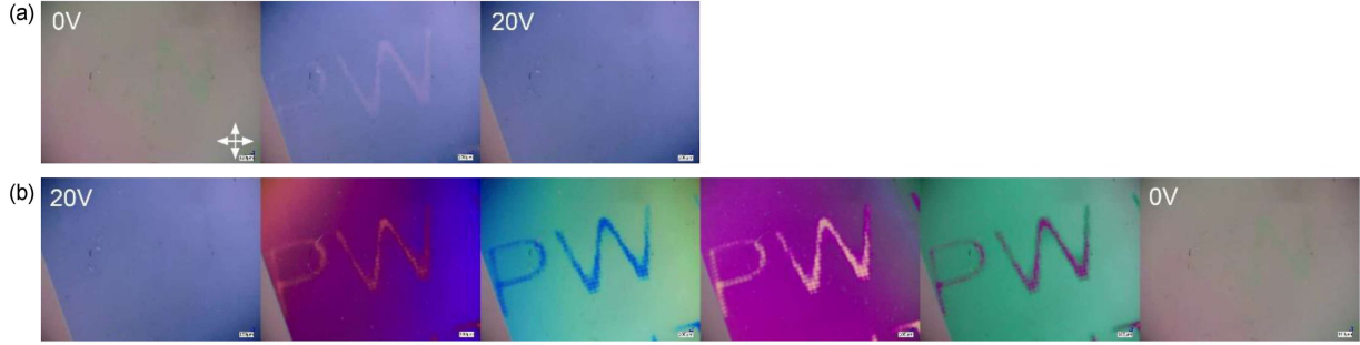
Fig. 2. Polymerized NLC-based sample observed under a polarizing microscope. The sample is examined during switching on with 20 V (a) and then during relaxation after the voltage is switched off (b). The ON and OFF states are marked with 20 V and 0 V, respectively. In each row, the images between the ON and OFF states show the sample during the switching process, which is further demonstrated in Fig. 3.
