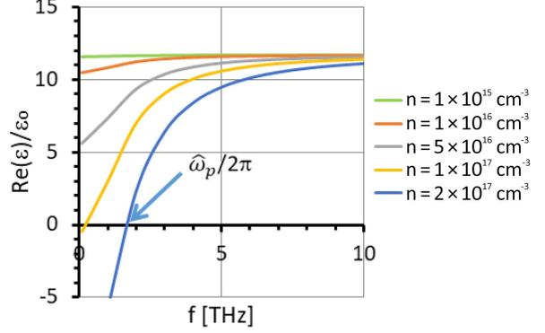
Fig. 1. Real part of the dielectric function (normalized to the permittivity of vacuum) vs frequency for moderately phosphorus-doped silicon at 300 K ( $\tau = 0.1$  ps). For all concentrations below ca.  $1 \times 10^{17} \text{ cm}^{-3}$ ,  $\text{Re}(\varepsilon)$  is positive.
