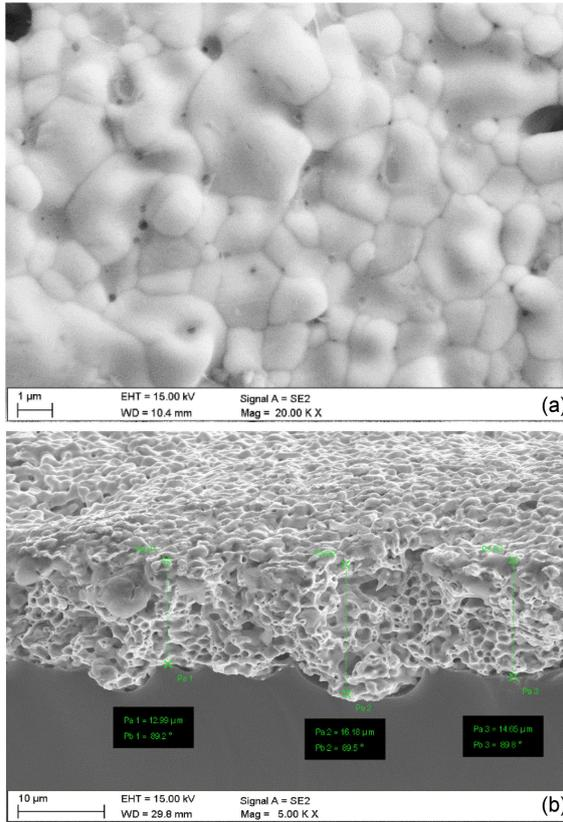
Fig. 9. Topography (a) and cross-section (b) of the front electrode (collecting path) of the chosen sample (SEM).
