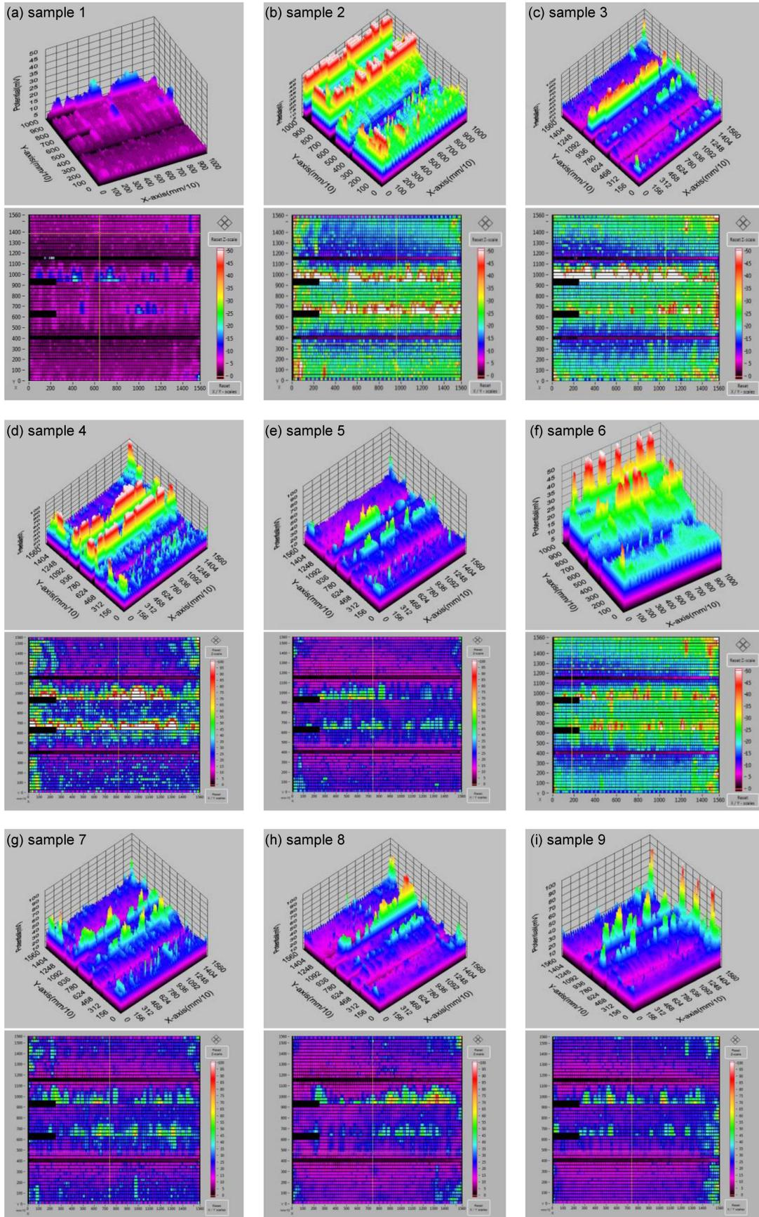
Fig. 4. Original measurement printout of the resistance distribution in the form of a 3D and 2D images for 9 solar cells.
