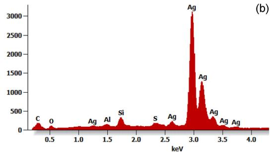
Fig. 11. (a) Front electrode topography of sample no. 6 and (b) EDS microanalysis from the X1 area.
