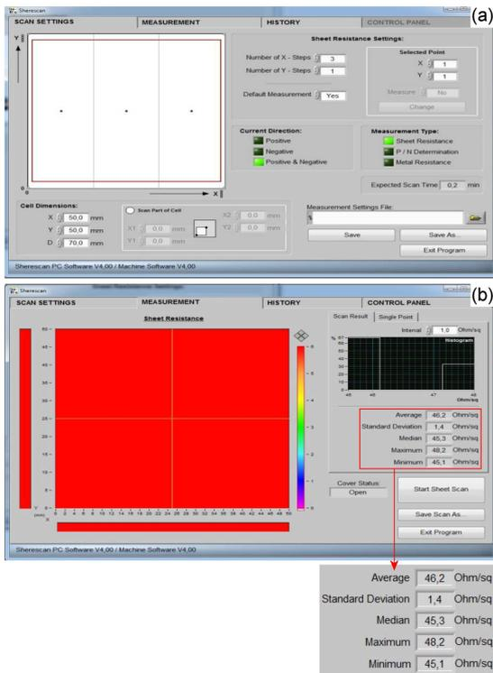
Fig. 6. View of the (a) scanning settings tab and (b) sheet resistance measurement tab.
