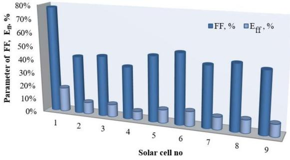
Fig. 8. Comparison of photovoltaic cells in terms of FF and  $E_{ff}$ .
