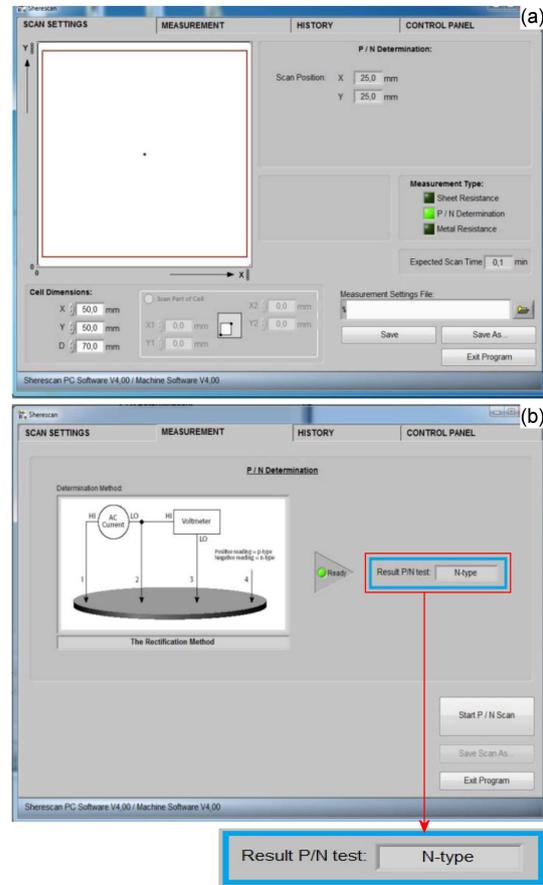
Fig. 7. Measurement of the recognition of the p/n conductivity type of a solar cell: (a) view of the scanning settings tab, (b) view of the measurement tab along with the obtained result.
