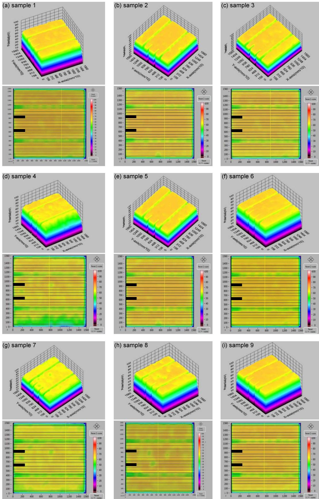
Fig. 5. Original printout of the measurement of the short-circuit current distribution on the surface of all solar cells in the form of a 3D and 2D image.
