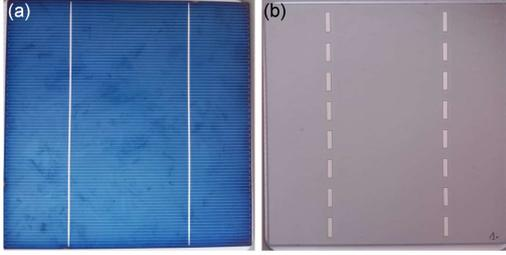
Fig. 3. Multicrystalline solar cell: (a) front, (b) back (example).
