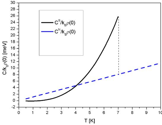
Fig. 3. Dependence of the specific heat of the superconducting and normal state on temperature.
