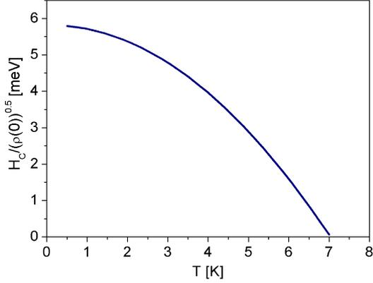
Fig. 5. Thermodynamic critical field as a function of temperature.
