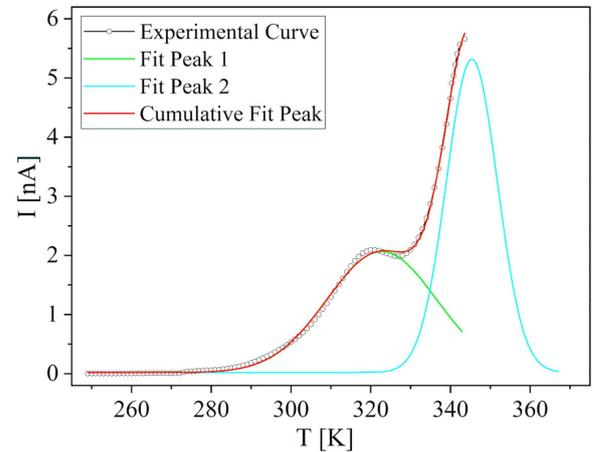
Fig. 2. Current spectrum of the thermally stimulated discharge for clathrate SBA-15(IL<sub>2</sub>) and approximation by a superposition of Gaussian functions.
