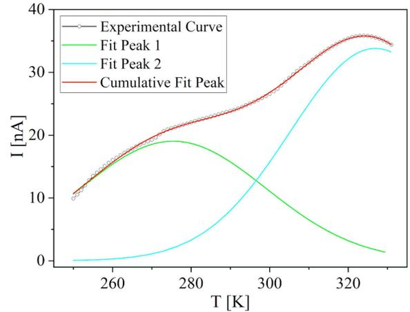
Fig. 1. Current spectrum of the thermally stimulated discharge for clathrate GaSe(IL<sub>1</sub>) and approximation by a superposition of Gaussian functions.
