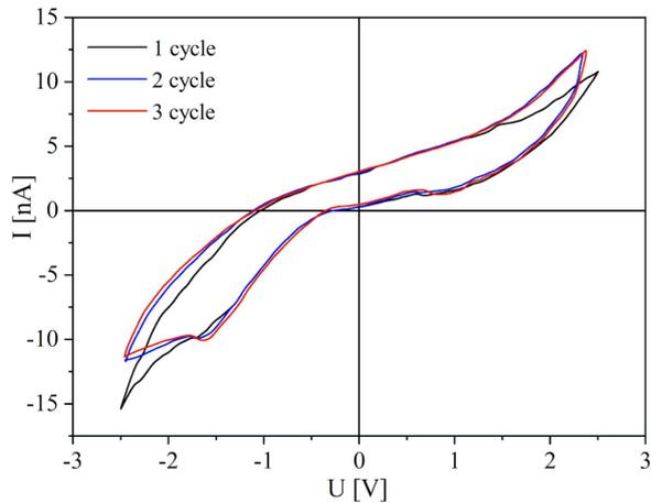
Fig. 4. The  $V$ - $A$  characteristics for clathrate  $\text{SBA-15}\langle\text{IL}_2\rangle$ .
