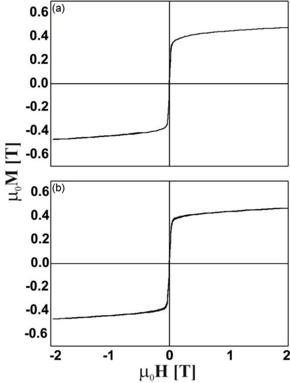
Fig. 3. Static hysteresis magnetic loops for the tested alloys: (a)  $\text{Fe}_{65}\text{Nb}_5\text{Y}_5\text{Hf}_5\text{B}_{20}$ , (b)  $\text{Fe}_{65}\text{Nb}_5\text{Y}_6\text{Hf}_4\text{B}_{20}$ .
