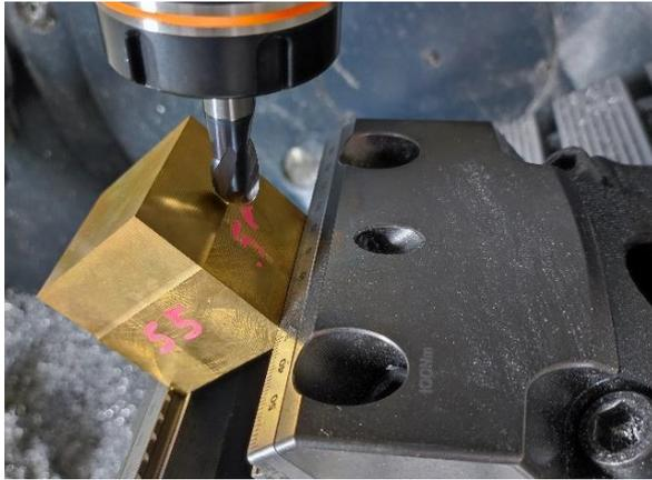
Fig. 1. Machining of MO58 brass alloy sample.
