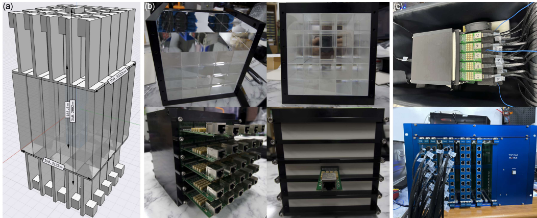
Fig. 7. (a) Schematic representation of the overall KAPAE II detector. (b) Assembly process of the KAPAE II detector. (c) Detector connected to the DAQ system.
