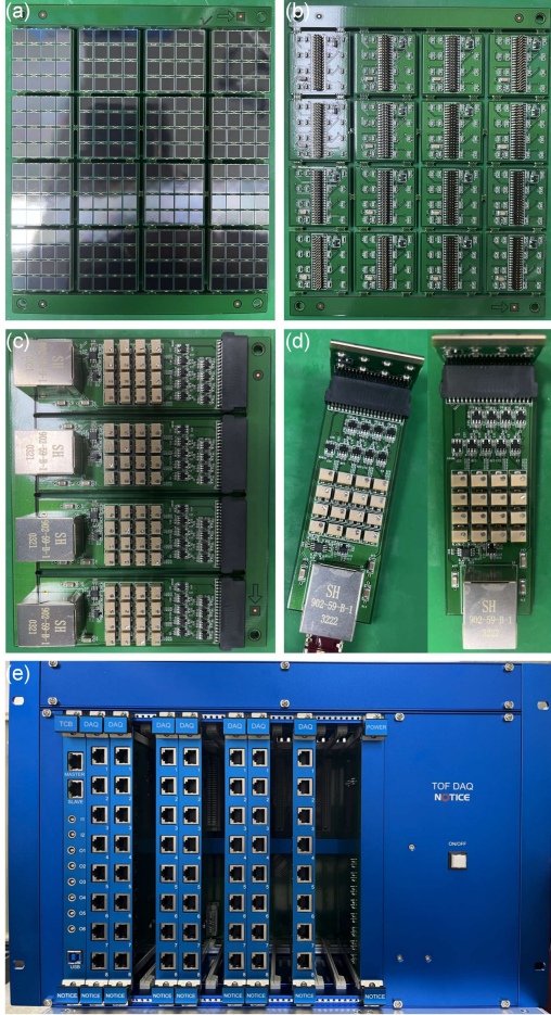
Fig. 5. (a) Front view and (b) back view of the custom 4 \times 4 array SiPM. (c) Preamp directly coupled to the SiPM. (d) Combined view of the array SiPM and preamp. (e) The custom DAQ system capable of connecting up to 64 channels.
