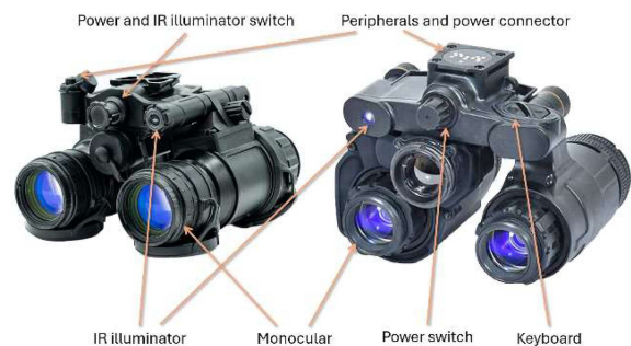
Fig. 2. Distinguished functional blocks on the example of night vision goggles PVS-31D from Armasight and PSQ-42 from L3Harris, see [14].
