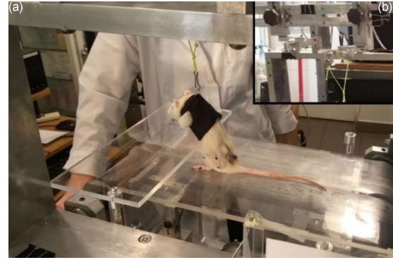
Fig. 6. Adapting the rat to the research station; (a) the rat is standing on the treadmill and connecting to the BWS, (b) knobs of the BWS system adjustment.
