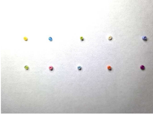
Fig. 2. Mass standards made of mother-of-pearl.
