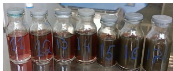
Fig. 1. Colloidal silver solutions obtained by chemical reduction of \text{AgNO}_3 using ChS and glucose. The numbering of colloidal solutions is: 11 — colloidal solution after 2 h from the beginning of infusion; 12 — after 4 h; 13 — after 6 h; 14 — after 12 h; 15 — after 24 h; 16 — after 30 h; 17 — after 48 h.
