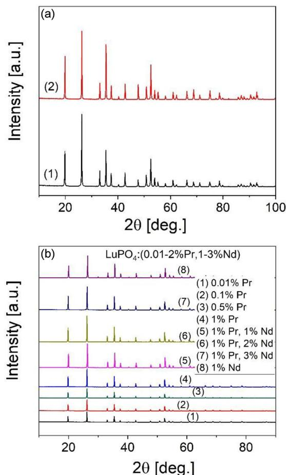
Fig. 2. XRD patterns of (a) (NCr)  $\text{LuPO}_4$  synthesized without CTAB and annealed at  $1000^\circ\text{C}$  (1) and  $1200^\circ\text{C}$  (2); (b)  $\text{LuPO}_4\text{:Pr:Nd}$  microcrystals synthesized by a solid-state method.
