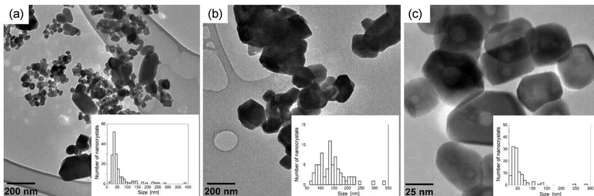
Fig. 3. TEM images of the pure (NCr)  $\text{LuPO}_4$  (a–c) and histograms of their distribution (in the insets). The sample of (NCr)  $\text{LuPO}_4$  was synthesized without CTAB and annealed at  $1000^\circ\text{C}$  (a) and after that at  $1200^\circ\text{C}$  (b). The sample in (c) was synthesized with CTAB and annealed at  $1000^\circ\text{C}$ .
