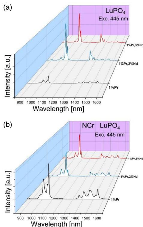
Fig. 7. NIR emission spectra of nano (b) and microcrystalline (a)  $\text{LuPO}_4$  excited at 445 nm recorded for Pr single-doped and Pr + Nd co-doped  $\text{LuPO}_4$ .
