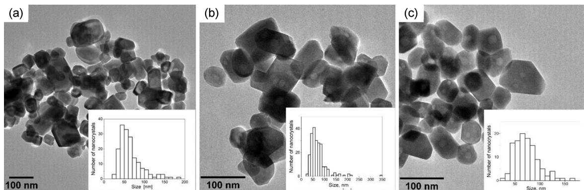
Fig. 5. TEM images of  $\text{LuPO}_4:1\%\text{Pr}$  (1–3%Nd) nanocrystals with the concentration of  $\text{Nd}^{3+}$  (1% (a), 2% (b), 3% (c)) in the solution. The samples were synthesized with CTAB and annealed at  $1000^\circ\text{C}$ .
