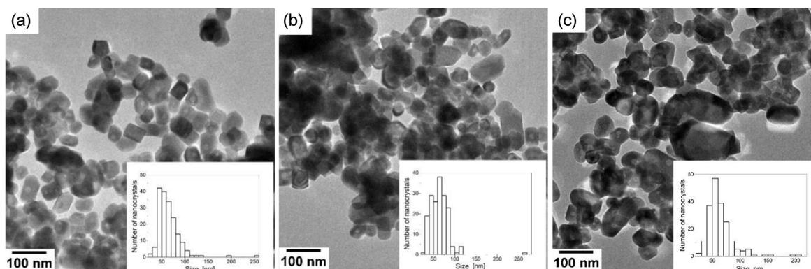
Fig. 4. TEM images of  $\text{LuPO}_4:\text{Pr}$  nanocrystals with different concentration of  $\text{Pr}^{3+}$  (0.5% (a), 1% (b), 2% (c)) in the solution. The samples were synthesized with CTAB and annealed at  $1000^\circ\text{C}$ .
