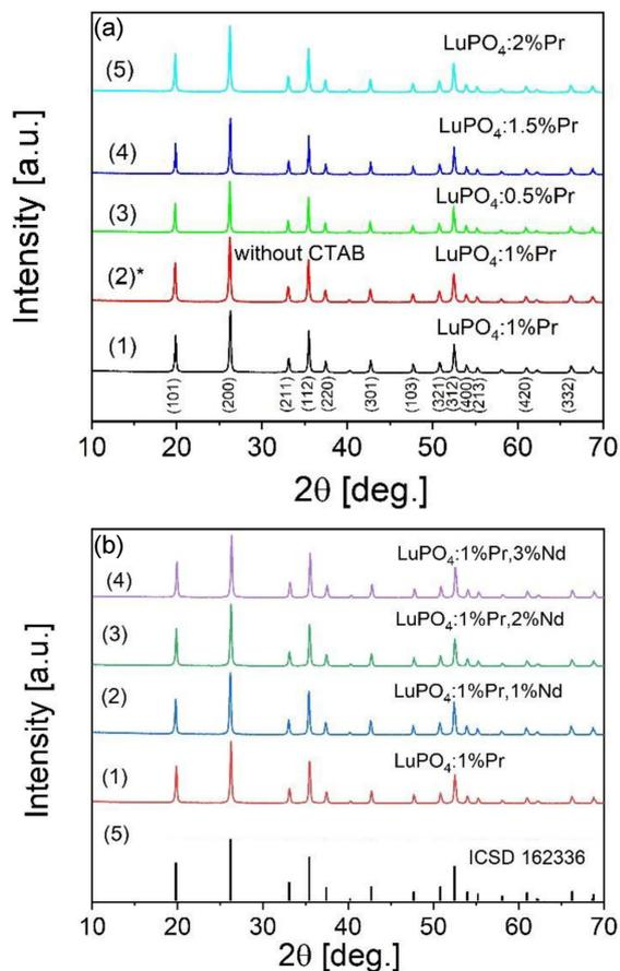
Fig. 1. XRD patterns of (NCr)  $\text{Lu}_{1-x-y}\text{Pr}_x\text{Nd}_y\text{PO}_4$  synthesized with different concentrations of  $\text{Pr}^{3+}$  and  $\text{Nd}^{3+}$  ions in the solutions. The samples 1, 3–5 (a) and 1–4 (b) were prepared with CTAB, but the sample 2\* (a) – without CTAB. The samples were annealed at  $1000^\circ\text{C}$ . The “ICSD 162336” spectrum of  $\text{LuPO}_4$  – spectrum 5.
