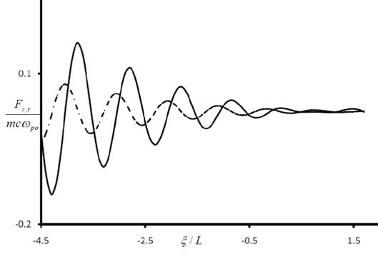
Fig. 1. Variation of the normalized axial  $F_z/(mc\omega_{po})$  (solid line) and transverse  $F_r/(mc\omega_{po})$  (dashed line) forces acting on a test electron within the pulse with  $\frac{\xi}{L}$  ( $x$ -axis) for  $a_o^2 = 0.9$ ,  $\lambda_p = 15.0 \mu\text{m}$ ,  $r_o = 15.0 \mu\text{m}$ ,  $r = 4.0 \mu\text{m}$ , and  $\omega_b/\omega = 0.5$ .
