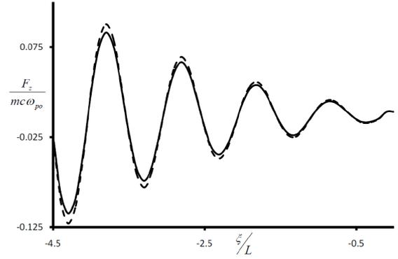
Fig. 4. Variation of the normalized axial force  $F_z/(mc\omega_{po})$  acting on an electron within the pulse with  $\xi/L$  for a quantum plasma (solid line) and for the classical case in the limit  $\hbar \rightarrow 0$  (dashed line).
