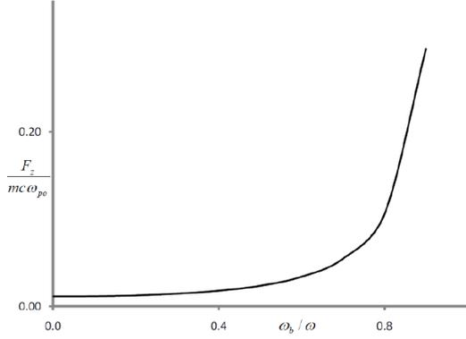
Fig. 3. Variation of the normalized axial force  $F_z/(mc\omega_{po})$  with normalized frequency  $\omega_b/\omega$  ( $x$ -axis) of the external magnetic field for  $a_o^2 = 0.9$ ,  $\lambda_p = 15.0 \mu\text{m}$ ,  $r_o = 15.0 \mu\text{m}$ ,  $r = 4.0 \mu\text{m}$ , and  $\xi/L = 4.0$ .
