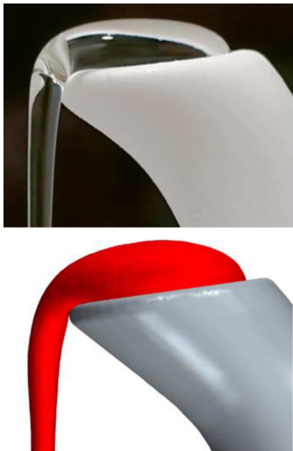
Fig. 13. Liquid flowing from superhydrophobic teapot spout (flow rate of 0.15 l/min).
