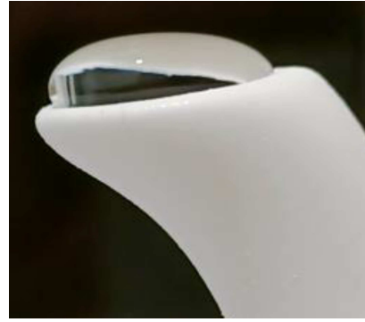
Fig. 12. The standing of the water before its discharge from the superhydrophobic spout.
