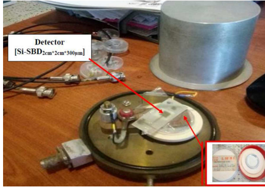
Fig. 3. Alpha spectrometry with ^{239}\text{Pu} standard source, bench test.
