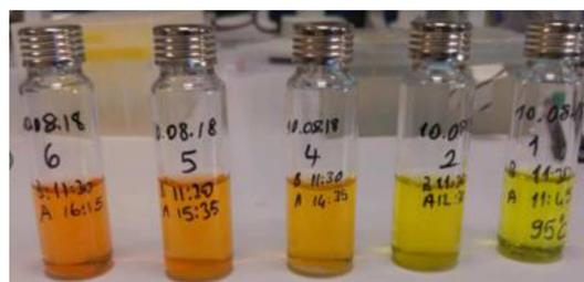
Fig. 4. CdTe QDs in aqueous solution with different sizes.
