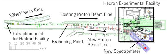
Fig. 2. Schematic view of Hadron Experimental Facility and a transfer beam line.
