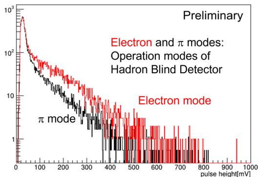
Fig. 5. Pulse height distributions of Lead Glass Calorimeter for electron candidates and  $\pi$  meson candidates.
