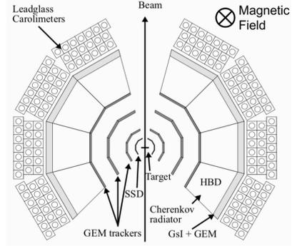
Fig. 3. Schematic view of the spectrometer.
