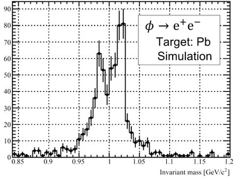
Fig. 1. Expected invariant mass spectrum of  $\phi \rightarrow e^+e^-$  for lead target and  $\beta\gamma$  of  $\phi$  less than 0.5 obtained using a Monte Carlo simulation including full detector simulations assuming a mass shift of 9%.
