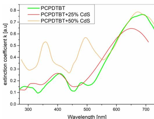
Fig. 4. Extinction coefficient spectral dispersion of PCPDTBT and its composites.
