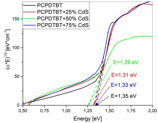
Fig. 2. Band gap width for PCPDTBT/CdS layers.
