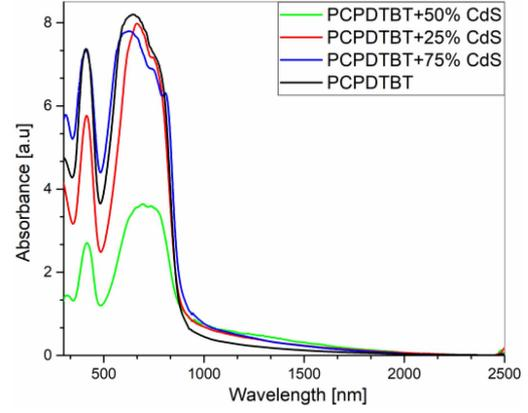
Fig. 1. Absorbance spectra for PCPDTBT/CdS nanoparticles films.
