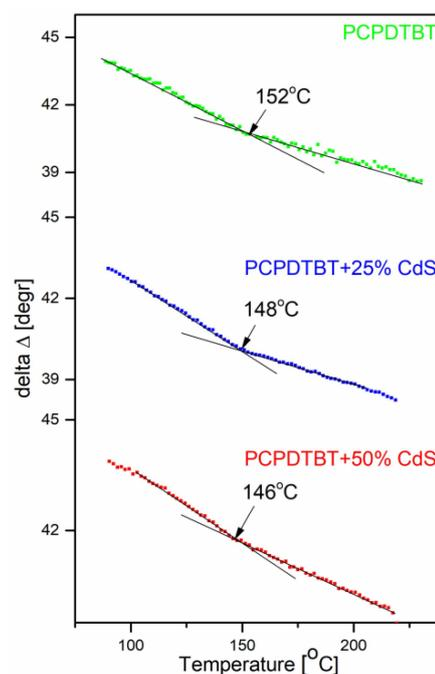
Fig. 5. Ellipsometric angle  $\Delta$  at  $\lambda = 930$  nm as a function of temperature.
