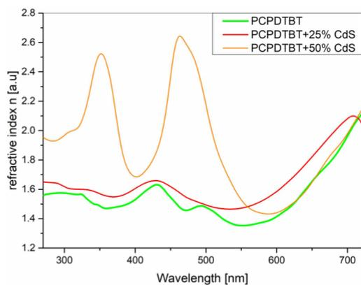
Fig. 3. Refractive index spectral dispersion of PCPDTBT and its composite films.
