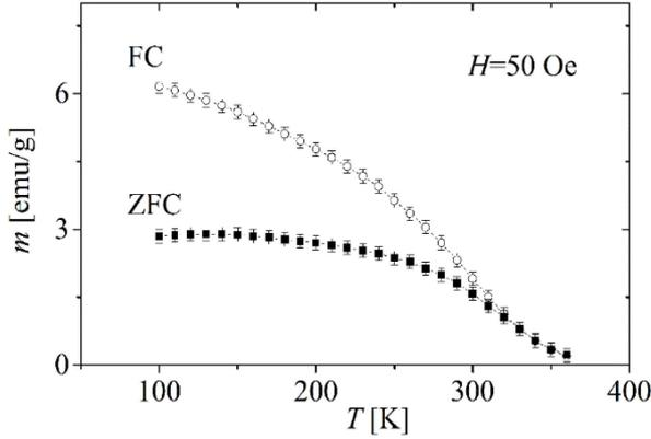
Fig. 3. Measurement data according to FC and ZFC protocols. Temperature dependence for magnetizations  $m_{FC}(T)$  and  $m_{ZFC}(T)$  measured in a field  $H = 50$  Oe.
