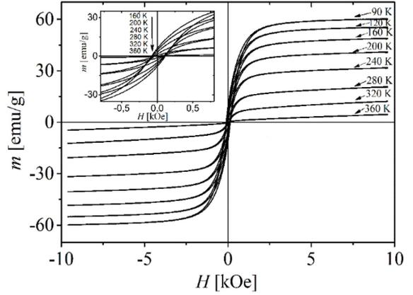
Fig. 1. Magnetization curves  $m(H)$  in the range of magnetic fields of  $\pm 10$  kOe. The inset shows parts of the hysteresis loops in the range of  $\pm 0.8$  kOe fields.
