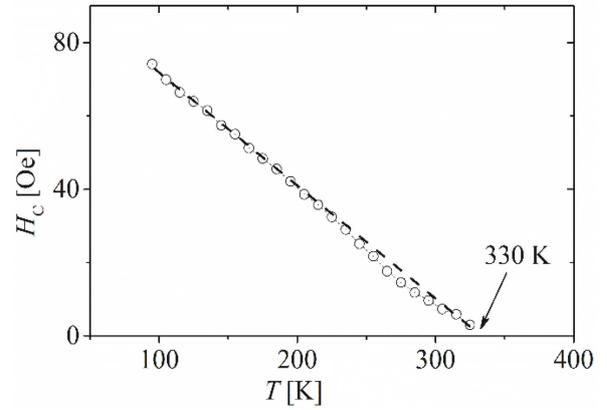
Fig. 2. Temperature dependence of the coercive force  $H_c(T)$ .
