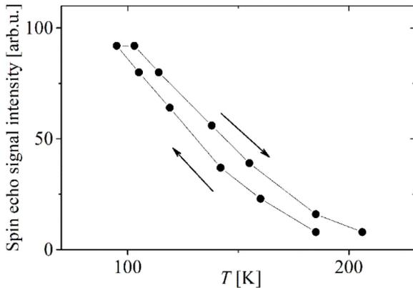
Fig. 4. Temperature dependence of the intensity of the  $^{139}\text{La}$  spin echo signal from the demagnetized LSMO nanopowder (measurements started from a high temperature).
