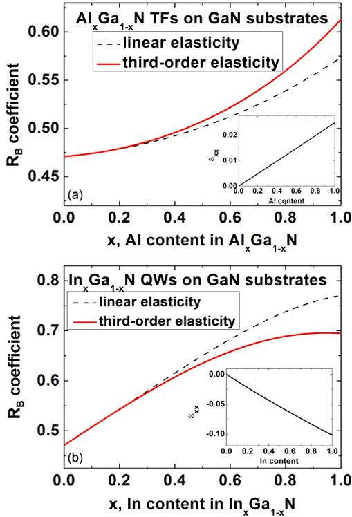
Fig. 4. The  $R_B$  coefficient for (a)  $\text{Al}_x\text{Ga}_{1-x}\text{N}$  TFs and (b)  $\text{In}_x\text{Ga}_{1-x}\text{N}$  QWs grown on GaN substrates as a function of chemical composition of the strained layers. Solid (dashed) lines correspond to the results obtained using third-order (linear) elasticity. The insets show  $\varepsilon_{xx}$  as a function of chemical composition of strained layers.
