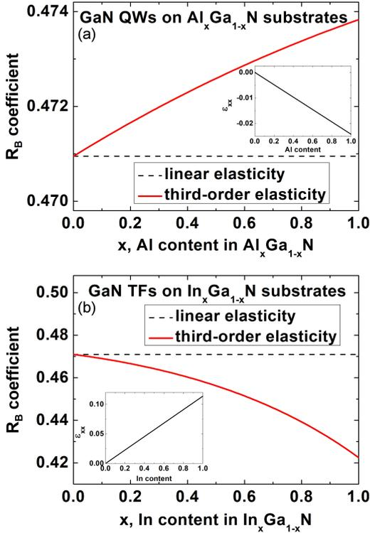
Fig. 2. The  $R_B$  coefficient for (a) GaN QWs grown on  $\text{Al}_x\text{Ga}_{1-x}\text{N}$  substrates and (b) GaN TFs grown on  $\text{In}_x\text{Ga}_{1-x}\text{N}$  substrates as a function of chemical composition of substrates. Solid (dashed) lines correspond to the results obtained using third-order (linear) elasticity. The insets show the in-plane strain  $\varepsilon_{xx}$  as a function of chemical composition of substrates.
