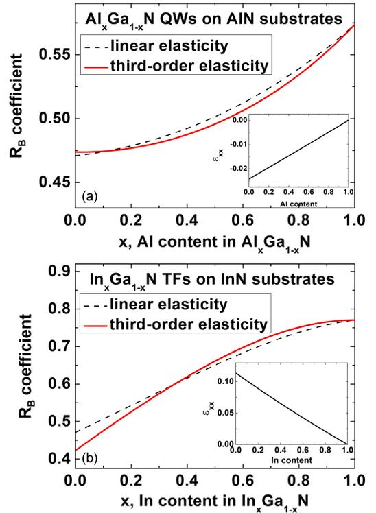
Fig. 5. The  $R_B$  coefficient for (a)  $\text{Al}_x\text{Ga}_{1-x}\text{N}$  QWs grown on AlN substrates and (b)  $\text{In}_x\text{Ga}_{1-x}\text{N}$  TFs grown on InN substrates (b) as a function of chemical composition of the strained layers. Solid (dashed) lines correspond to the results obtained using third-order (linear) elasticity. The insets show  $\varepsilon_{xx}$  as a function of chemical composition of strained layers.
