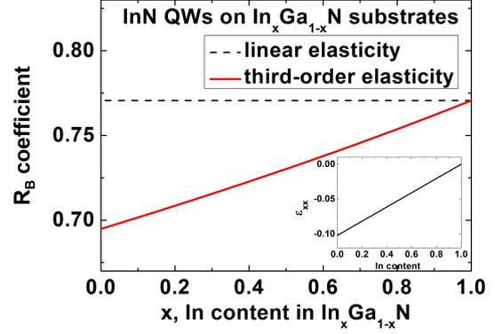
Fig. 3. The  $R_B$  coefficient for InN QWs as a function of In content in  $\text{In}_x\text{Ga}_{1-x}\text{N}$  substrates. Solid (dashed) line corresponds to the results obtained using third-order (linear) elasticity. The inset shows the in-plane strain  $\varepsilon_{xx}$  as a function of In content in  $\text{In}_x\text{Ga}_{1-x}\text{N}$  substrates.
