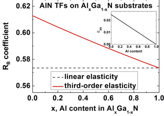
Fig. 1. The  $R_B$  coefficient for AlN TFs as a function of Al content in  $\text{Al}_x\text{Ga}_{1-x}\text{N}$  substrates. Solid (dashed) line corresponds to the results obtained using third-order (linear) elasticity. The inset shows the in-plane strain  $\varepsilon_{xx}$  as a function of Al content in  $\text{Al}_x\text{Ga}_{1-x}\text{N}$  substrates.
