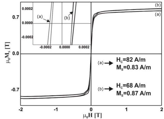
Fig. 2. Static magnetic hysteresis loops for tested alloys in solidified state: (a)  $\text{Fe}_{70}\text{Y}_5\text{Nb}_5\text{B}_{20}$ , (b)  $\text{Fe}_{70}\text{Y}_5\text{Nb}_5\text{Mo}_1\text{B}_{20}$ .
