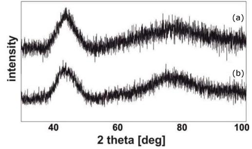
Fig. 1. X-ray diffraction patterns for the alloy samples: (a)  $\text{Fe}_{70}\text{Y}_5\text{Nb}_5\text{B}_{20}$ , (b)  $\text{Fe}_{70}\text{Y}_5\text{Nb}_5\text{Mo}_1\text{B}_{20}$ .
