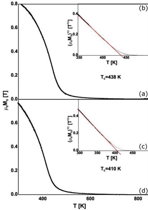
Fig. 3. Thermomagnetic curves for:  $\text{Fe}_{70}\text{Y}_5\text{Nb}_5\text{B}_{20}$  alloy: (a)  $\mu_0 M_S(T)$ , (b)  $\mu_0 M_S^{1/\beta}(T)$  and for  $\text{Fe}_{70}\text{Y}_5\text{Nb}_5\text{Mo}_1\text{B}_{20}$  alloys: (c)  $\mu_0 M_S(T)$ , (d)  $\mu_0 M_S^{1/\beta}(T)$ .
