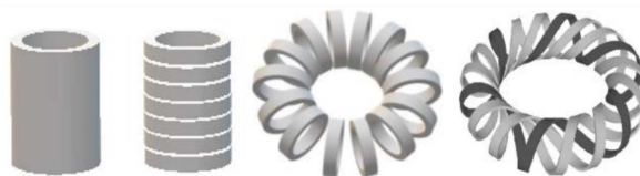
Fig. 3. Possible winding configuration for the SMES system.
