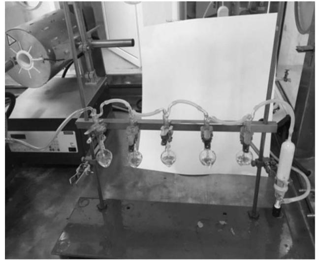
Fig. 2. Apparatus for C-14 and H-3 determination release in gas phase.
