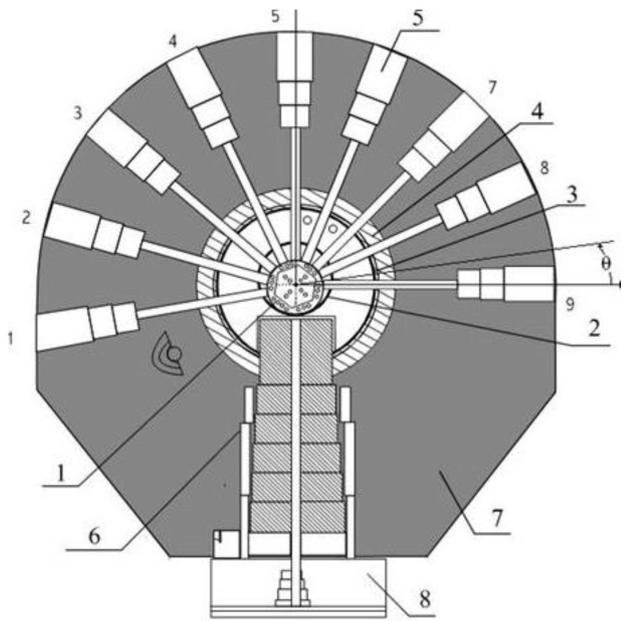
Fig. 1. Vertical cut-view through the VVR — S reactor and the movable thermal column, 1 — reactor core, 2 — median vessel, 3 — outer vessel, 4 — cast-iron rings, 5 — beam tubes, 6 — thermal column, 7 — biological shield, 8 — thermal column shielding.
