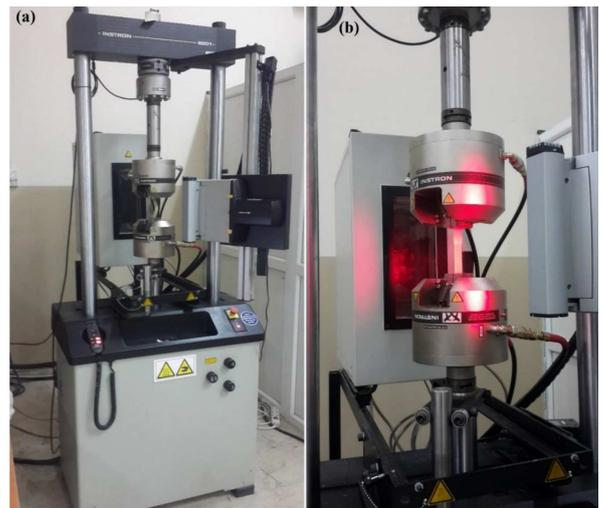
Fig. 3. (a) test equipment, Instron 8801, (b) mechanical testing of a composite specimen.
