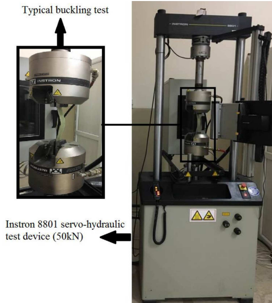
Fig. 2. Experimental setup of Instron 8801 for buckling test.
