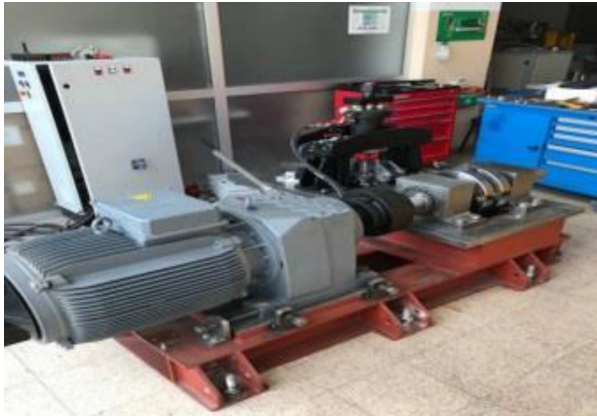
Fig. 2. Tribo-test rod wear setup.
