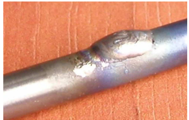
Fig. 6. Ti rod surfaced of Ti-Cu-Ni braze layer.
