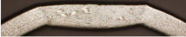
Fig. 1. Microstructure of cross-section of CuNi50 strip weld area.
