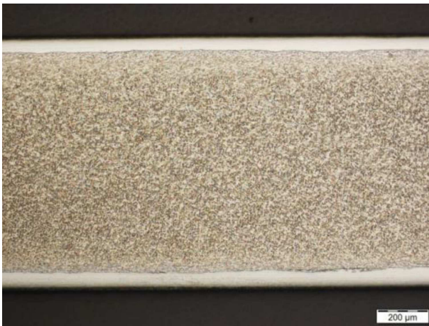
Fig. 5. Microstructure of longitudinal section of Ti/CuNi composite wire diameter 1.2 mm.
