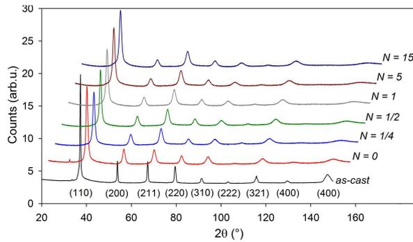
Fig. 2. The development of X-ray diffraction patterns for HfNbTaTiZr alloy during HPT straining for various number of HPT revolutions  $N$ .
