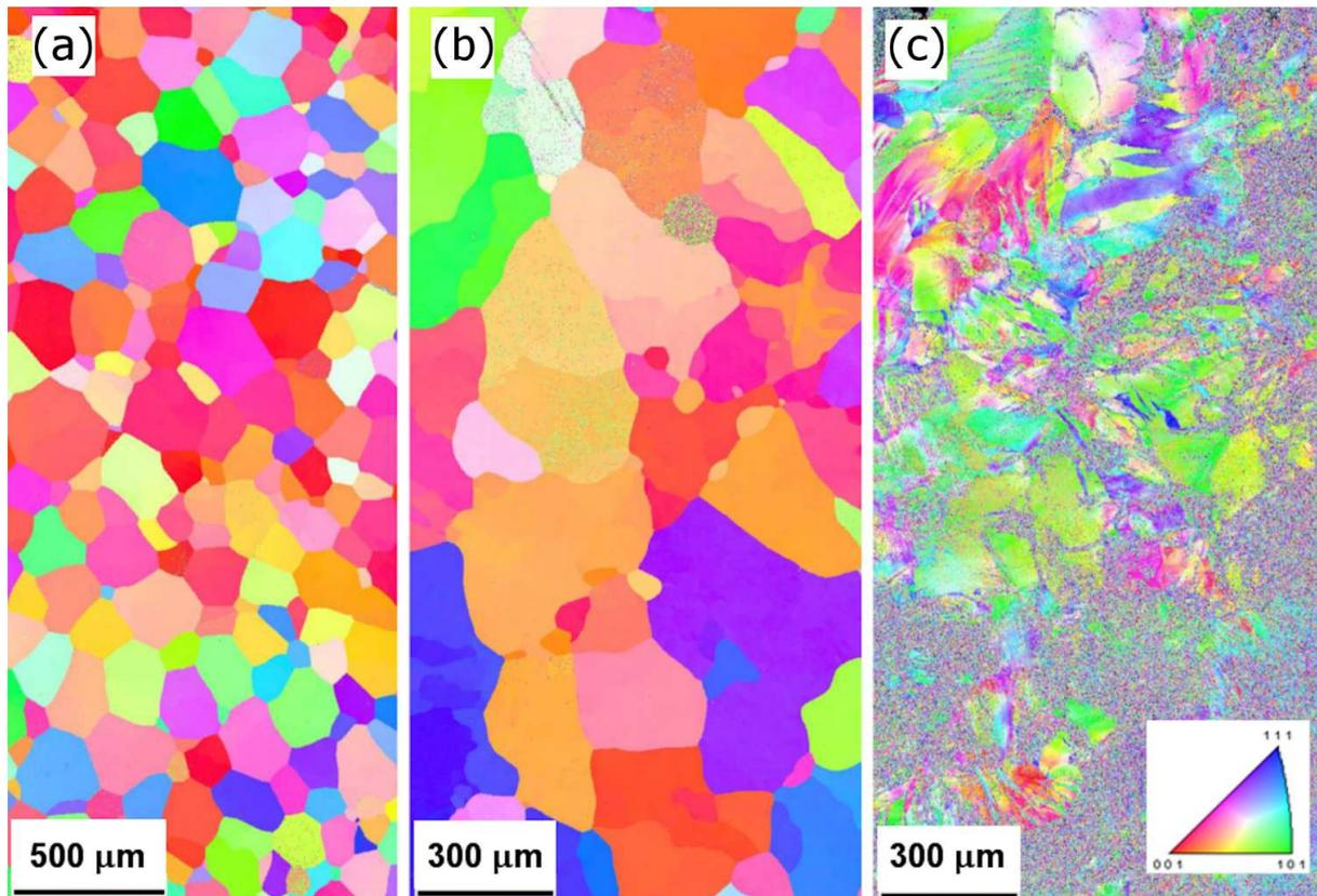
Fig. 1. EBSD maps of HfNbTaTiZr alloy (a) as-cast sample (b) sample compressed by high pressure of 2.5 GPa without any torsion deformation (number of HPT revolutions  $N = 0$ ) (c) HPT-deformed sample  $N = 1/2$ . The EBSD map was measured in the centre of the HPT-deformed sample.
