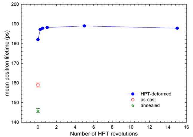
Fig. 4. The mean positron lifetime for HfNbTaTiZr alloy subjected to HPT straining. The PAS measurements were always performed in the centre of the sample disc.
