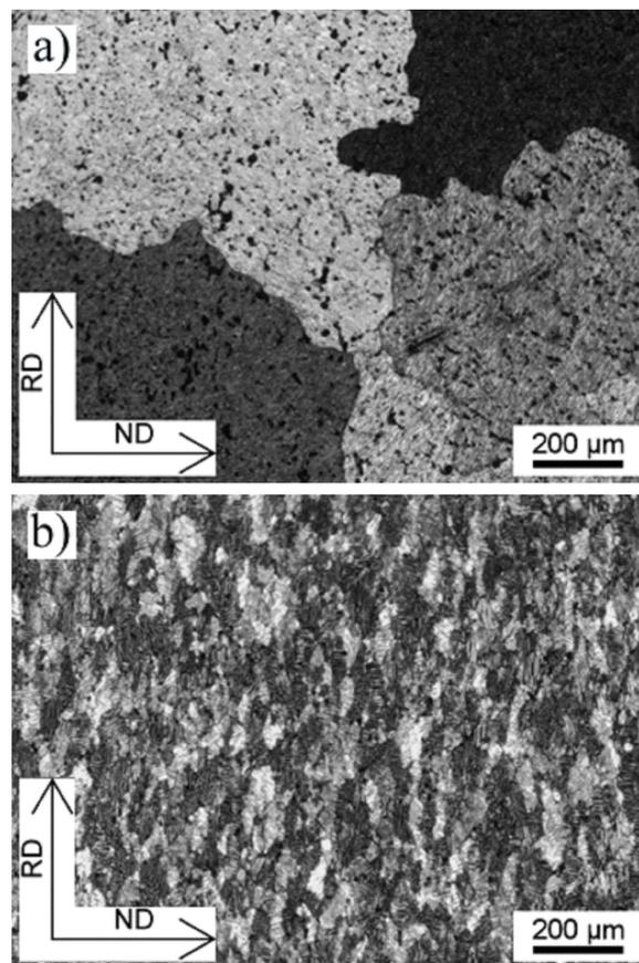
Fig. 5. Influence of  $\text{Al}_3(\text{Sc,Zr})$  particles on grain coarsening during isochronal annealing up to 550 °C. Coarse grains in Al-Mg (a) and stable structure Al-Mg-Sc-Zr (b) alloys.
