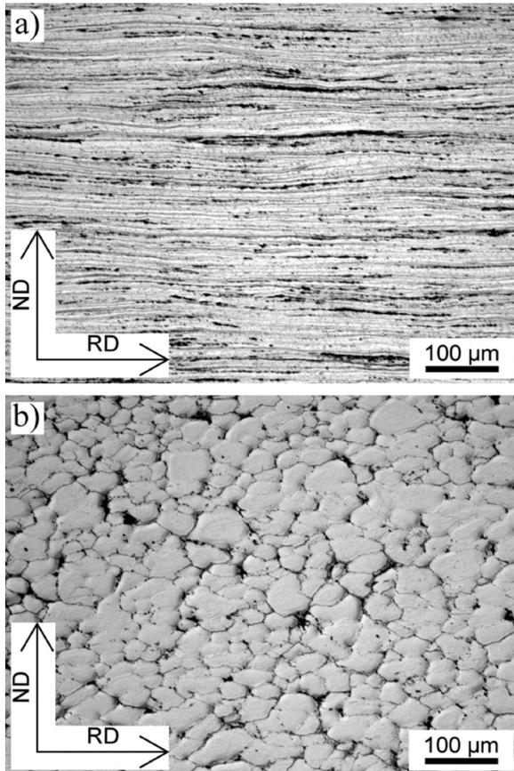
Fig. 1. Elongated flat grains in DC cast (a) and TRC (b) 5 mm thick strips prepared from Al-Mg-Sc-Zr alloy.
