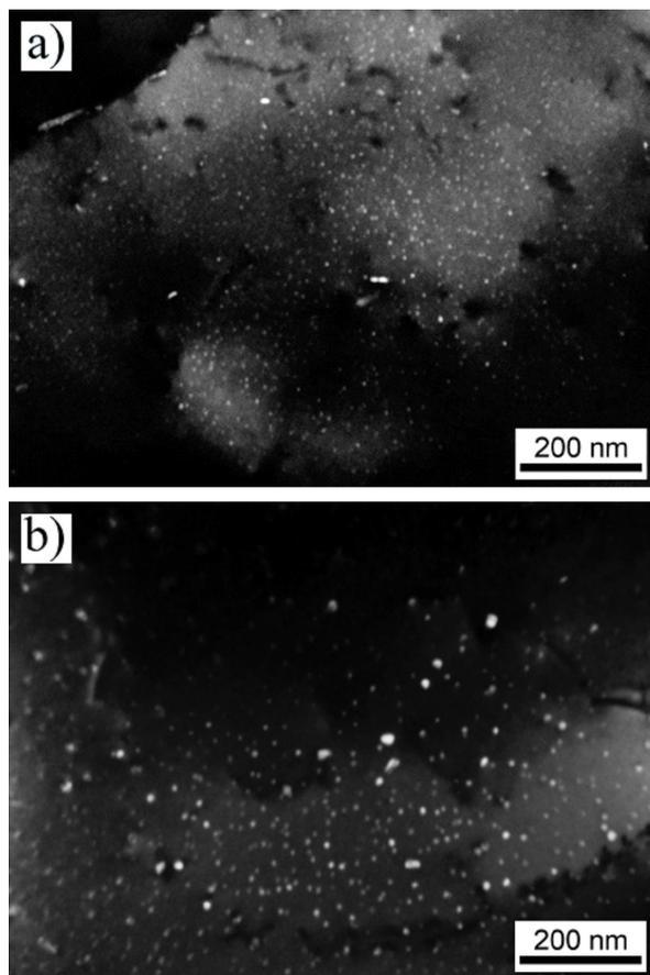
Fig. 4. Dark field TEM images of  $\text{Al}_3(\text{Sc,Zr})$  particles viewed near the  $[100]$  Al zone axis in TRC Al-Mg-Sc-Zr alloy after isothermal annealing at 300 (a) and 400 °C (b) for 8 h.
