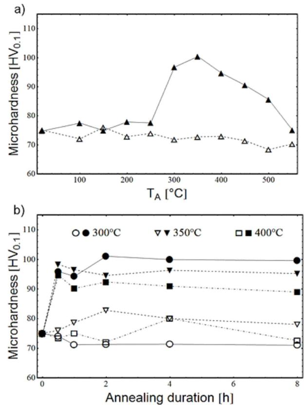
Fig. 3. Evolution of microhardness in TRC Al-Mg (empty symbols) and Al-Mg-Sc-Zr (full symbols) alloys during isochronal (a) and isothermal (b) annealing.
