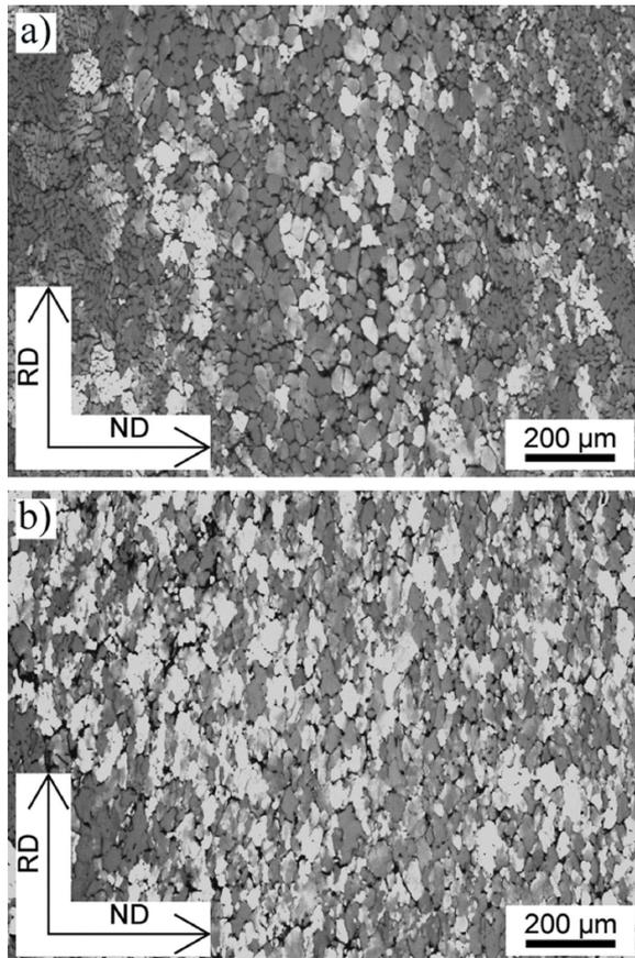
Fig. 2. Microstructure of TRC Al-Mg (a) and Al-Mg-Sc-Zr (b) alloys near the central part of the strip.
