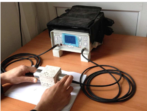
Fig. 2. Ultrasonic Pundit pulse generator device used for P-wave measurements.
