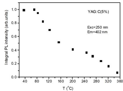
Fig. 5. Integral PL intensity of the YAG:C(5%) ceramics as a function of temperature.
