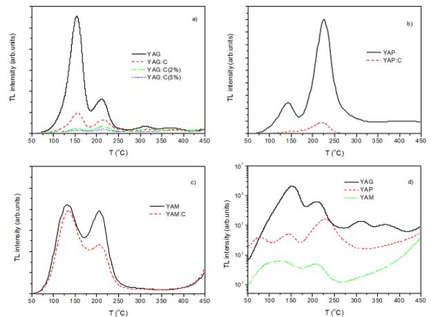
Fig. 6. Typical thermal glow curves of the studied ceramic samples registered just after  $\beta$ -irradiation at room temperature. Heating rate 4 °C/s.
