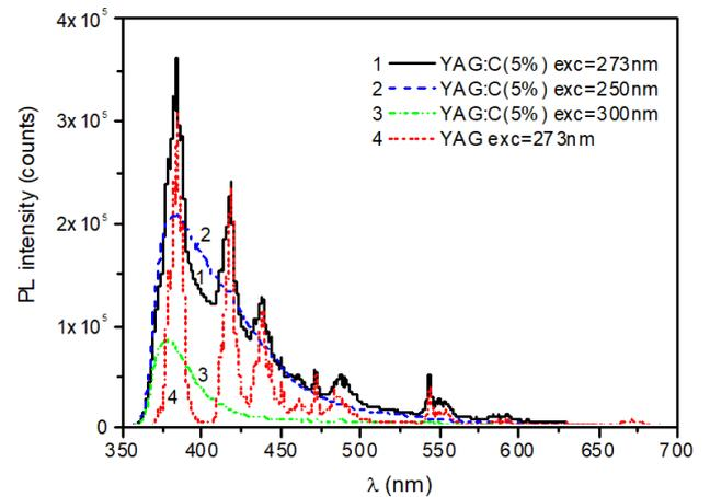
Fig. 2. Room temperature PL spectra of YAG (a) and YAG:C (b) ceramic samples at different wavelength of UV excitation.
