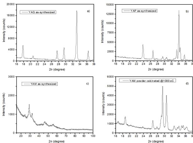
Fig. 1. X-ray diffraction patterns of the studied powder samples.
