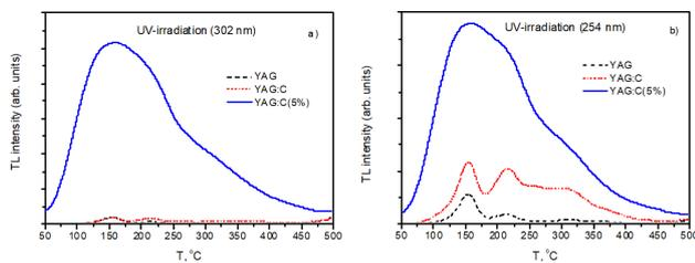
Fig. 7. Thermal glow curves of YAG and YAG:C ceramic samples registered just after UV light exposure at room temperature. Heating rate 4 °C/s.
