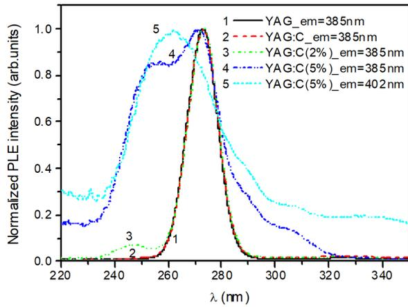
Fig. 3. Room temperature PLE spectra of YAG and YAG:C ceramic samples registered for different emission wavelengths.
