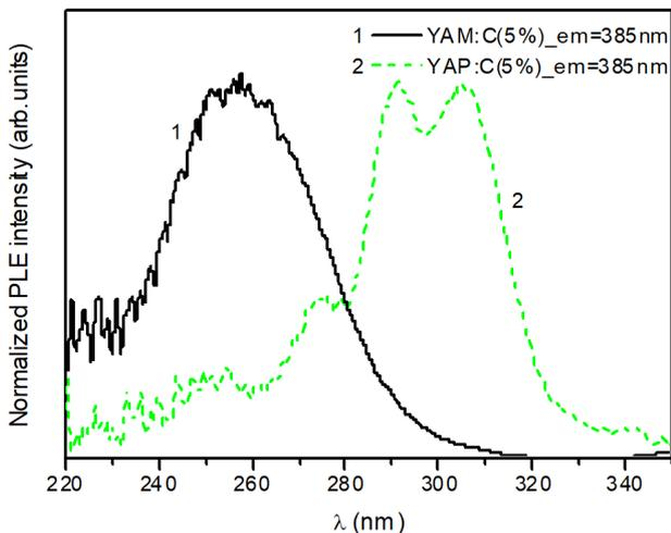
Fig. 4. Room temperature PLE spectra of YAP:C and YAM:C ceramic samples.
