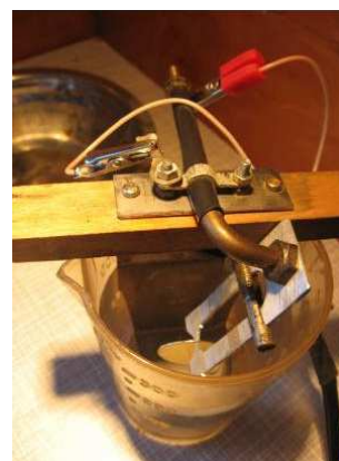
Fig. 1. Electrochemical cell with a U-shaped cathode.
