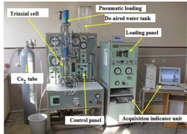
Fig. 1. The dynamic triaxial test system.
