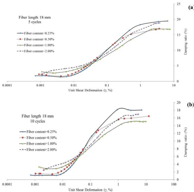
Fig. 7. Damping ratio vs strain values after (a) 5th and (b) 10th loading cycles.
