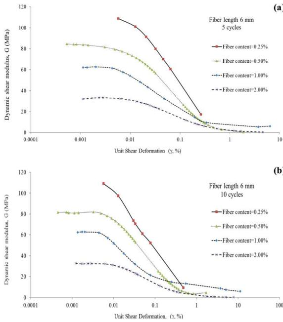
Fig. 2. Dynamic shear modulus vs strain values after (a) 5th and (b) 10th loading cycles.
