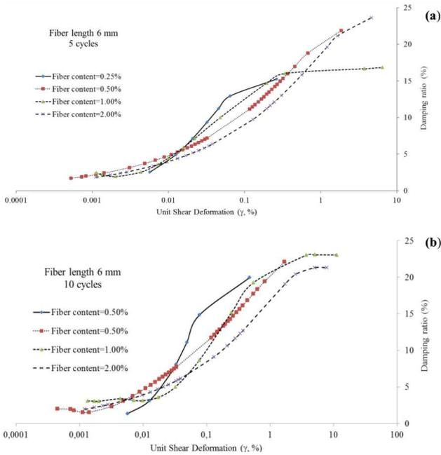
Fig. 3. Damping ratio vs strain values after (a) 5th and (b) 10th loading cycles.
