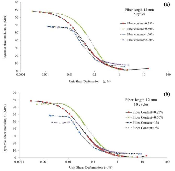
Fig. 4. Dynamic shear modulus vs strain values after (a) 5th and (b) 10th loading cycles.
