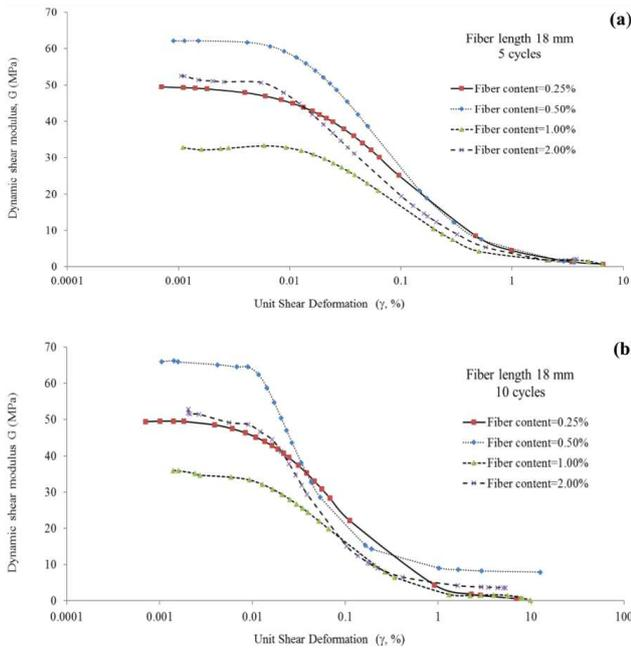
Fig. 6. Dynamic shear modulus vs strain values after (a) 5th and (b) 10th loading cycles.
