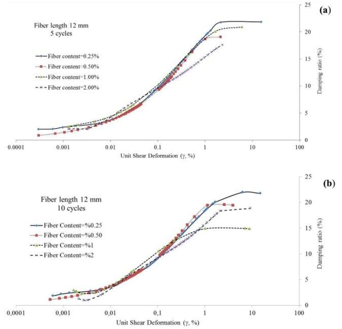
Fig. 5. Damping ratio vs strain values after (a) 5th and (b) 10th loading cycles.
