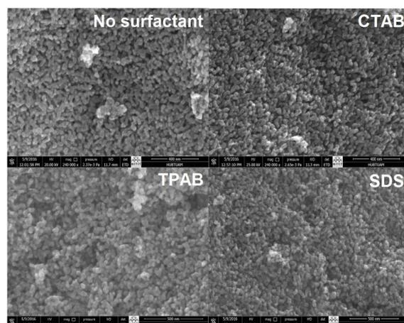
Fig. 3. FESEM micrograph of  $\text{SnO}_2$  nanoparticles by different surfactant assisted.
