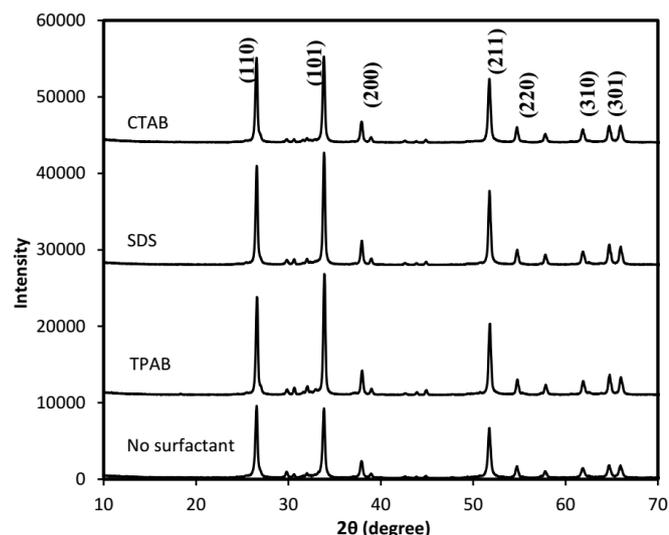
Fig. 1. XRD patterns of  $\text{SnO}_2$  nanoparticles by different surfactant assisted.
