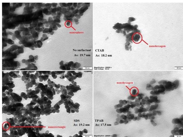
Fig. 4. TEM images of SnO<sub>2</sub> nanoparticles by different surfactant assisted.
