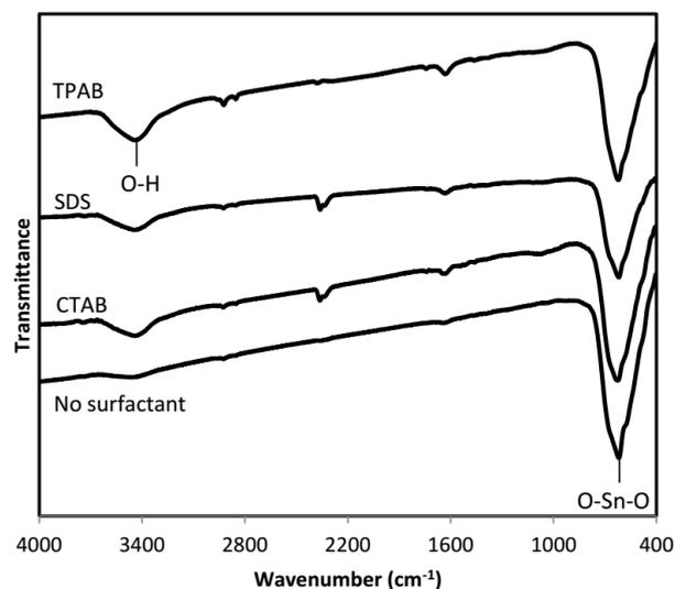
Fig. 2. FTIR spectra of  $\text{SnO}_2$  nanoparticles by different surfactant assisted.
