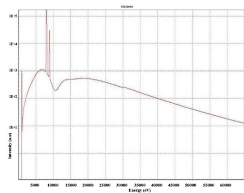
Fig. 4. K_{\alpha 1} and K_{\beta 1} peaks of pure Cu.
