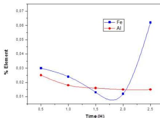
Fig. 4. Effect of H<sub>2</sub>SO<sub>4</sub> acid on percentages of iron and aluminium in Chlef sand.
