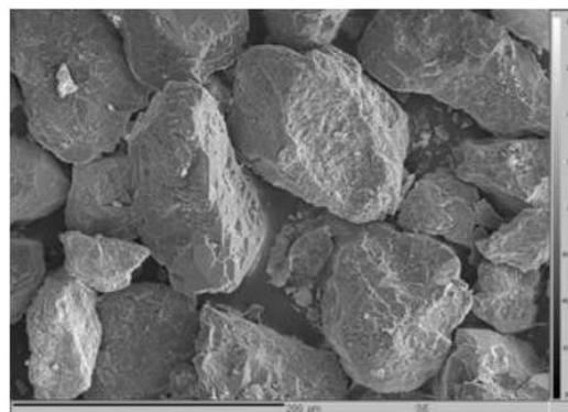
Fig. 6. Scanning electron micrograph of Chlef sand before leaching test.
