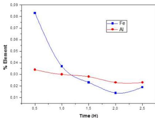
Fig. 5. Effect of H<sub>3</sub>PO<sub>4</sub> acid on percentages of iron and aluminum in Chlef sand.
