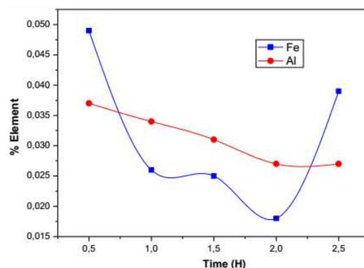
Fig. 3. Effect of H<sub>2</sub>C<sub>2</sub>O<sub>4</sub> acid on percentages of iron and aluminium in Chlef sand.
