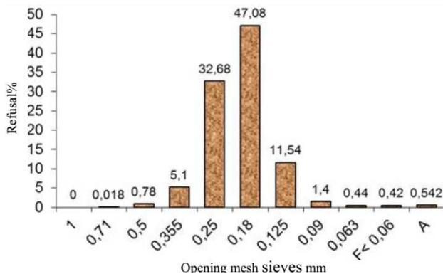
Fig. 1. Histogram representation of granulometric analysis of Chlef sand.
