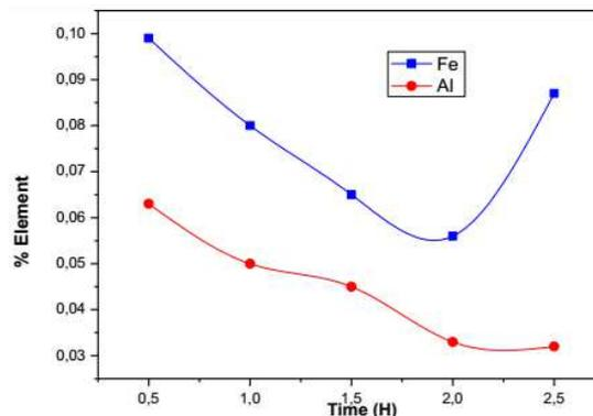
Fig. 2. Effect of HNO<sub>3</sub> acid on percentages of iron and aluminium in Chlef sand.
