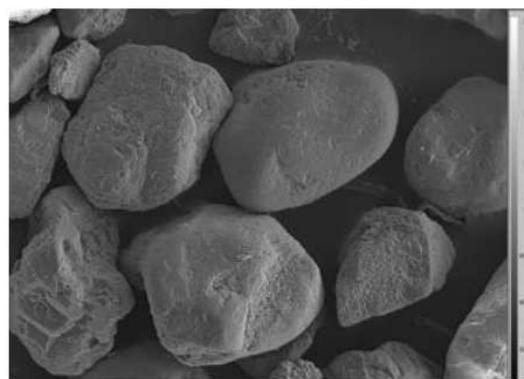
Fig. 7. Scanning electron micrograph of Chlef sand after leaching test.
